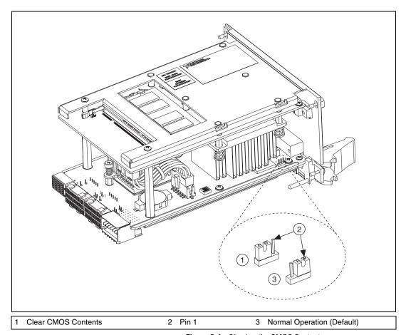
Figure 5-1. Clearing the CMOS Contents
